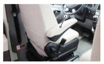
3. Pull the swivel lock lever (3) (located near the base of the seat) to the left, and swivel the seat slowly toward the center line of the motorhome to prevent damage to the seat, door panel and post.
