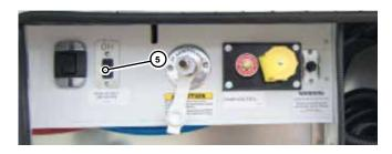
2. Do not attempt to manually light the furnace. The furnace does not have a pilot light. It is ignited by a direct spark ignition system.
