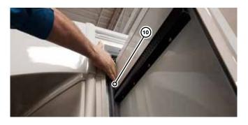
12. Push in the slide out room until fully retracted, keeping both sides of the slide out level with the coach while retracting.
