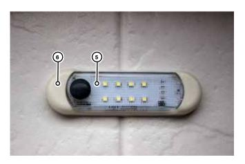
**NOTE:** This is a sealed LED unit and must be replaced as complete unit.
