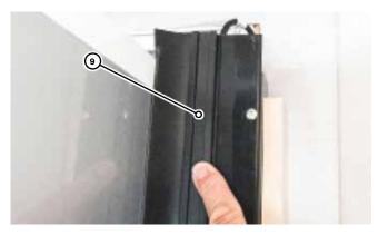
10. Locate the mounting screw on the ride side of the slide out and remove the screw.
