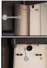
Push in the slide out room until fully retracted, keeping both sides of the slide out level with the coach while retracting.
