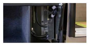
When shore power or generator power is absent, the inverter can be switched on and used to supply 120 volt AC power to the microwave, entertainment center, and any outlets being marked as inverted. No other receptacles will have power. The 2000 watt inverter has an internal 80 amp battery charger. Once the inverter has accepted the AC input power, Charge Mode will begin. It is not possible to turn off this charge mode.
