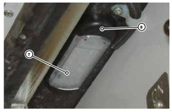
**NOTE:** This is a sealed LED unit and must be replaced as complete unit.
