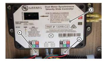
3. Unplug both motor electrical connectors (3 & 4) from the control module 2.
