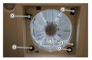
**NOTE:** The roof vent must be open at least 3 inches (76 mm) or the internal safety switch will prevent the fan from operating.
